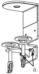
2. Place Vertical Assembly on Base (b). Make sure the External Tube is loosely secured by lining up cut-out with guide inside Base (c).
